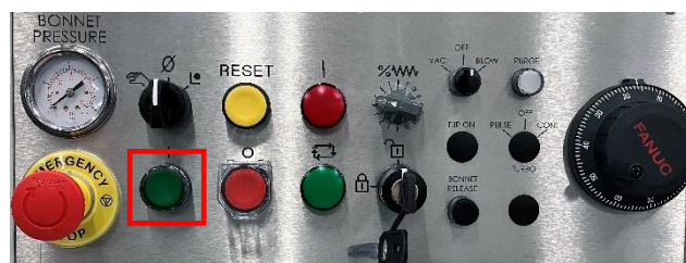
Figure 17 - CNC Drives ON switch
